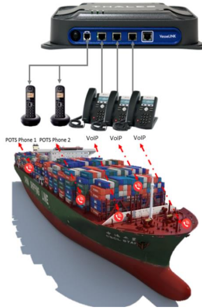
Figure 2-2 Local Communications via PBX Functionality
