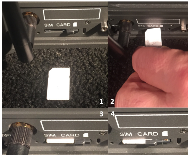
Figure 2-7 Installing SIM Card and Engaging the Lock
