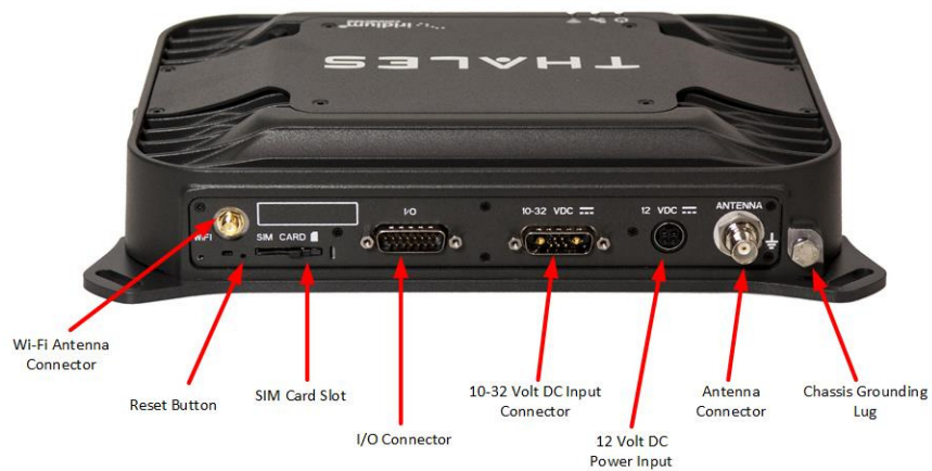
Figure 1-5 Terminal Unit (TU) Back Panel Detail
