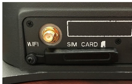
Figure 2-8 Secure the SIM Card Cover
