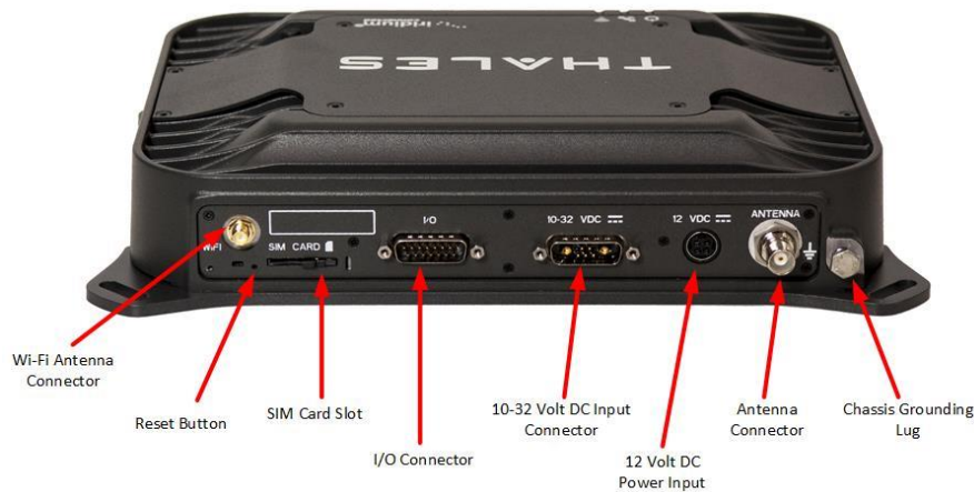
Figure 2-7 Terminal Unit (TU) Back Panel Detail
