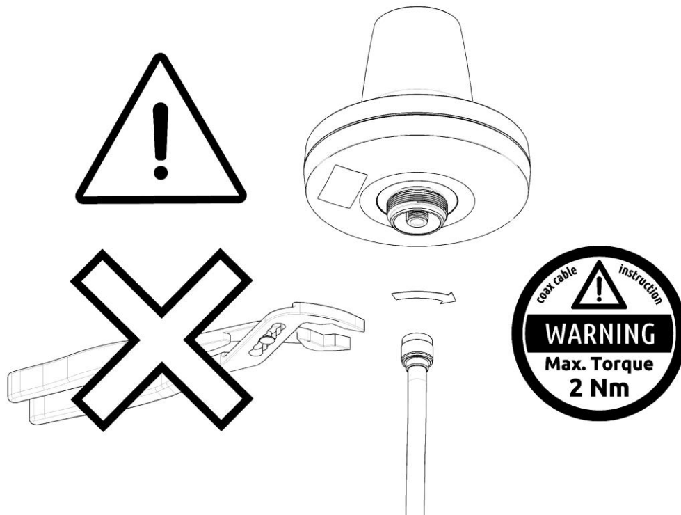
Figure 11: Connecting the coaxial cable N connector to the LT-3130 Antenna Unit
