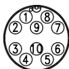
Figure 38: AUX connector (pin out)
