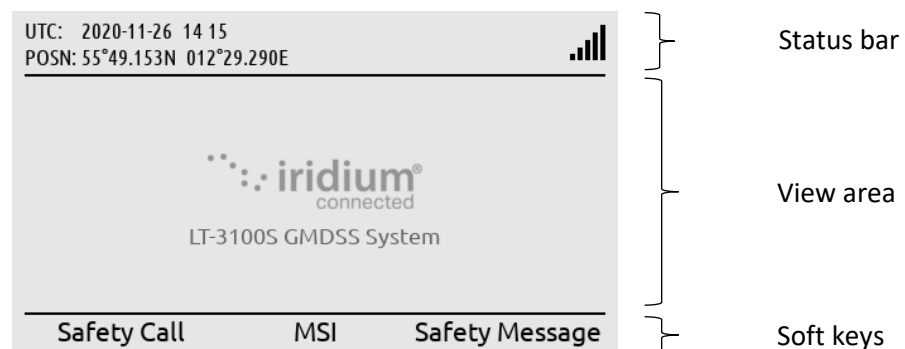
Figure 59: LT-3110S Control Unit (display sections)
