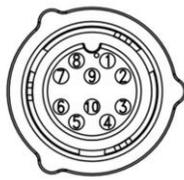
Figure 38: AUX cable (pin out)
