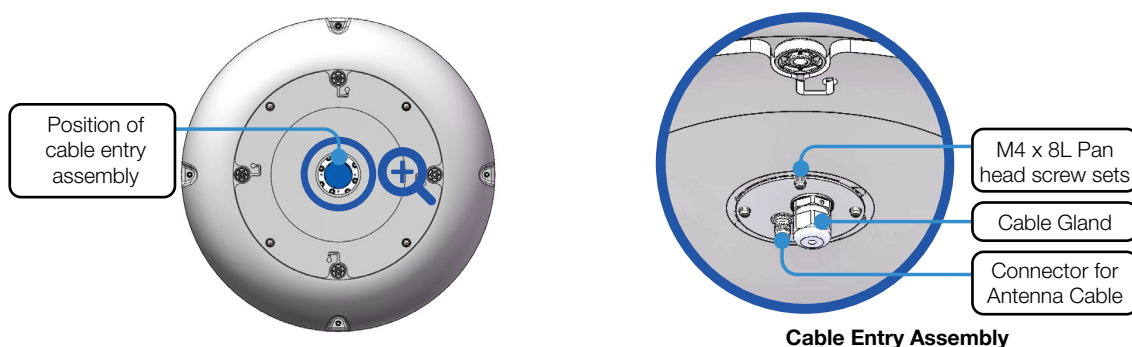
Figure 57: Attaching Position of Cable Entry
