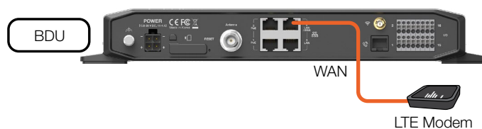
Figure 40: BDU to Device Cable Connection using WAN Port
