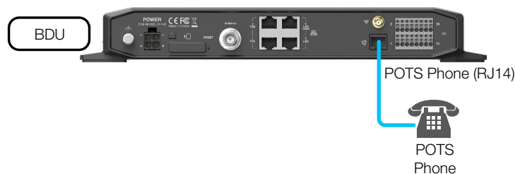
Figure 41: BDU to POTS Phone (RJ14) Cable Connection
