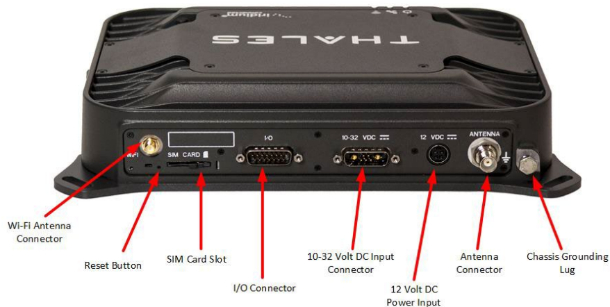
Figure 2-7 Terminal Unit (TU) Back Panel Detail
