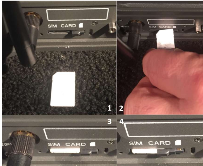
Figure 3-4 Installing SIM Card and Engaging the Lock
