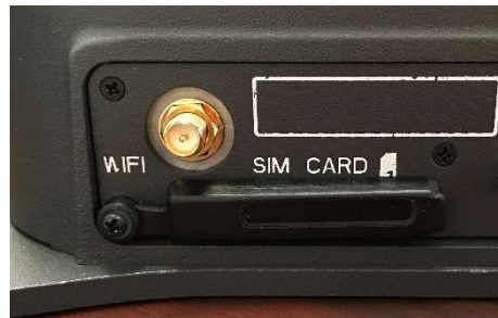
Figure 3-5 Secure the SIM Card Cover
