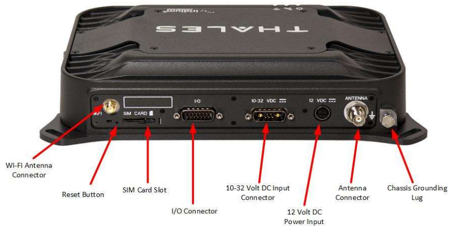
Figure 2-7 Terminal Unit (TU) Back Panel Detail
