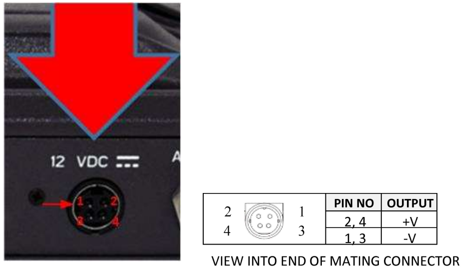
Figure 7-3 12V Input and Mating Connector Detail
