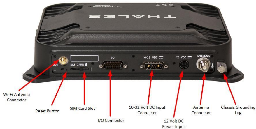
Figure 2-7 Below Deck Unit (BDU) Back Panel Detail
