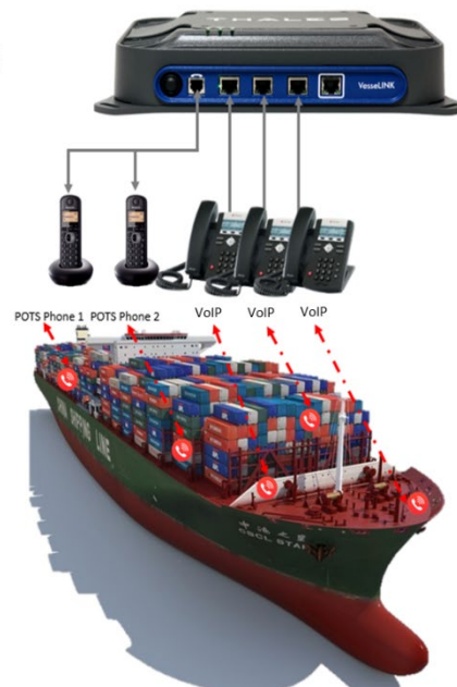
Figure 2-2 Local Communications via PBX Functionality
