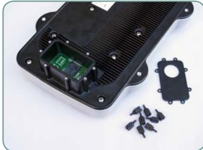
SABRE™ Ranger V1 Terminal Connector cover and thumb-screws
